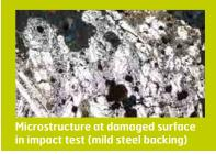
Under lab impact testing, the microstructure of the damaged surface of Duroxite $^{\rm m}$  101 exhibits some plastic deformation, but the primary carbides are not worn significantly. It shows better impact resistance with the Hardox 450 backing plate compared to mild steel.
